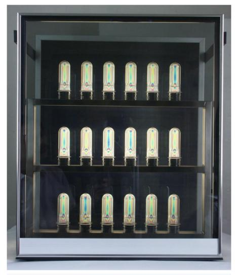
Standard model holds 18 piece (6 each level) of Preforms for 16 ounce or 600 ml Bottles. Other configurations and fixture sizes are specified at time of ordering More or less fixtures in a single inspection pass depending on size of Preforms
